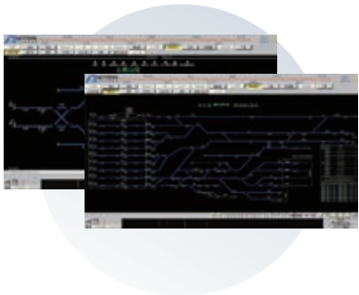
Automatic Train Supervision (ATS) System
