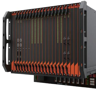
The ETS-SGM adopts the HiaGuard SIS (Safety Instrumented System) as its platform, which is developed by HollySys for the safety field of industrial automation and realizes emergency shutdown. HiaGuard is certified by TÜV (Rheinland Industrie Service GmbH) and meets SIL3 safety-related applications as defined by IEC 61508 (2010), and the safety-grade protection unit is a triple modular redundant system.
