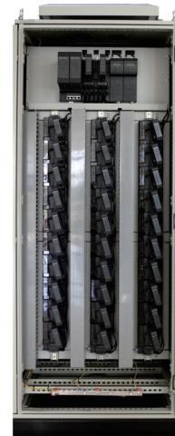
K series DEH (T800K) is a general-purpose system designed based on HOLLiAS ® MACS-K. It adopts fast master control, dedicated all-digital intelligent servo module, speed measurement protection module, CAN bus fast communication, and is equipped with a full range of I/O redundant modules to meet the stability requirements of different working conditions.
