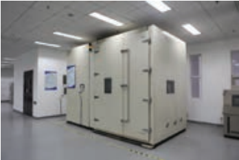
Stepping Cyclic Damp Heat Test
